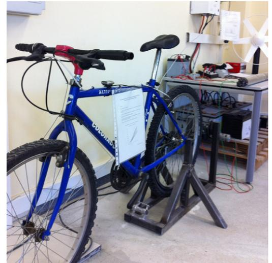
Experimental bicycle system for charging batteries.
